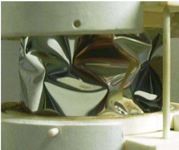
Fig. 5. View of the reducing atmosphere testing device after compression at low temperature.
